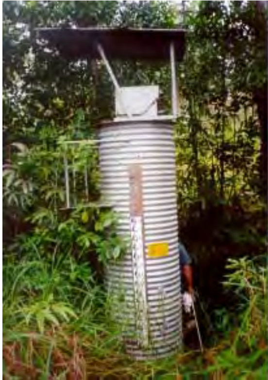
Figure 16 Gauging Tower at Blue Water Creek
